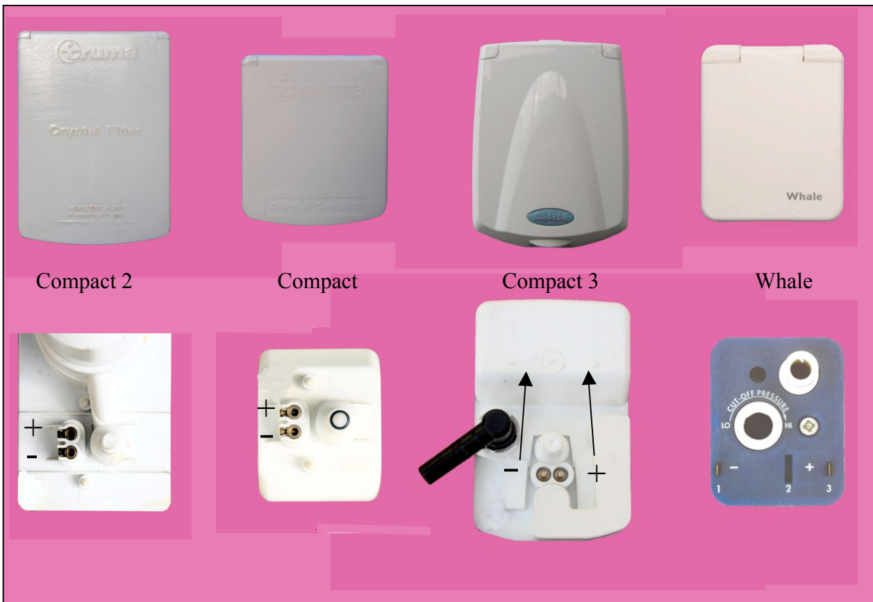
Pump housings viewed from inside caravan
